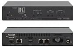
The VM-114H2C is a high-performance PoC switcher and distribution amplifier for HDMI and DGKat™ twisted pair signals. It reclocks and equalizes one of two selectable input signals (HDMI or DGKat twisted pair) and distributes it to two DGKat twisted pair and two HDMI outputs
